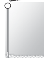
Noncutoff A luminaire light distribution where there is no candela limitation in the zone above maximum candela. (IESNA)
