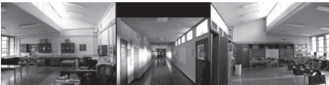
Left: Back to the Future 1952, Wilson School, first daylights the classrooms and secondly borrows the light to illuminate the corridors. A good daylighting design matches the daylight to the students' critical learning environments.
